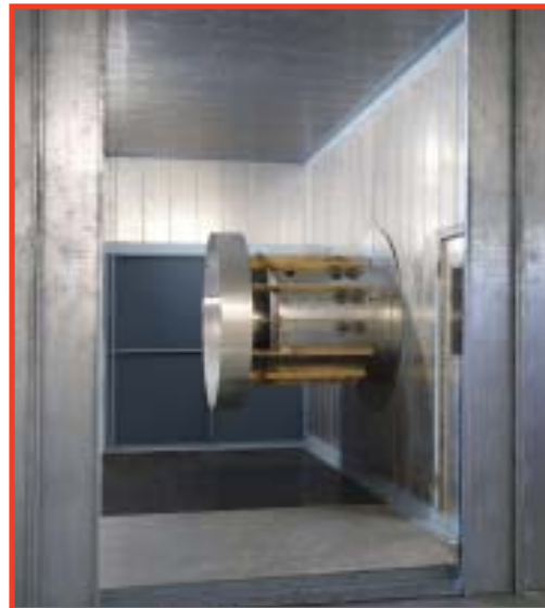
Test Duct Windbox with Burner Mock-up
