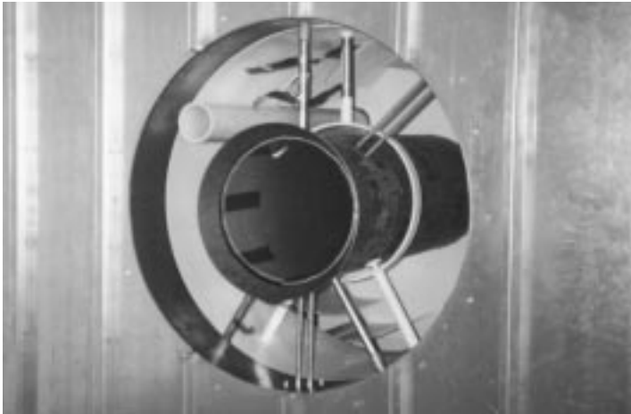
Figure 8 IBAM™ Probe Calibration Testing in AMC’s Wind Tunnel Facility
