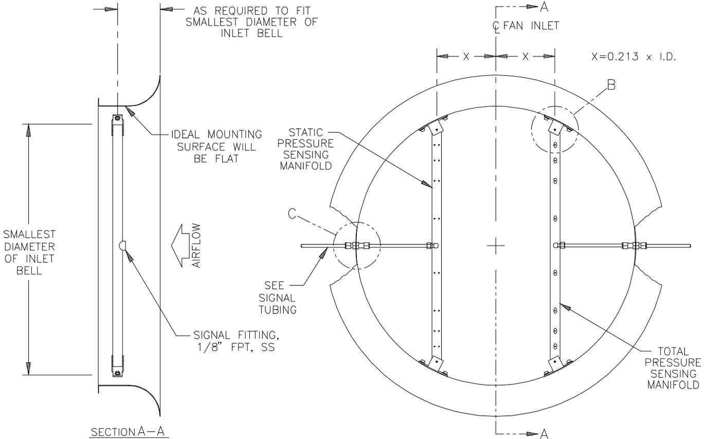
**Note:** When placing an order for a VOLU-probe/FI, be sure to state the minimum fan inlet diameter, not the fan model number nor the probe length. (The probe length will be approximately 0.905 the minimum inlet diameter for standard configurations.)
