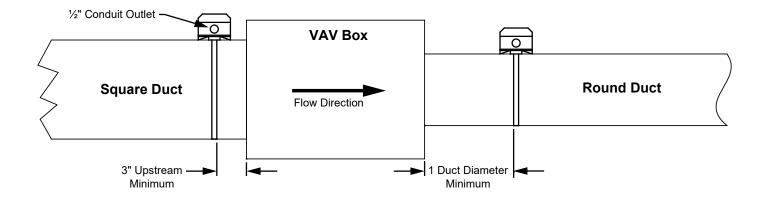
**VAV Installation Option 1:** Locate ELECTRA-flo/SD a minimum of 3" upstream of the VAV box, or 3" upstream of the pneumatic flow ring (remove the ring).
