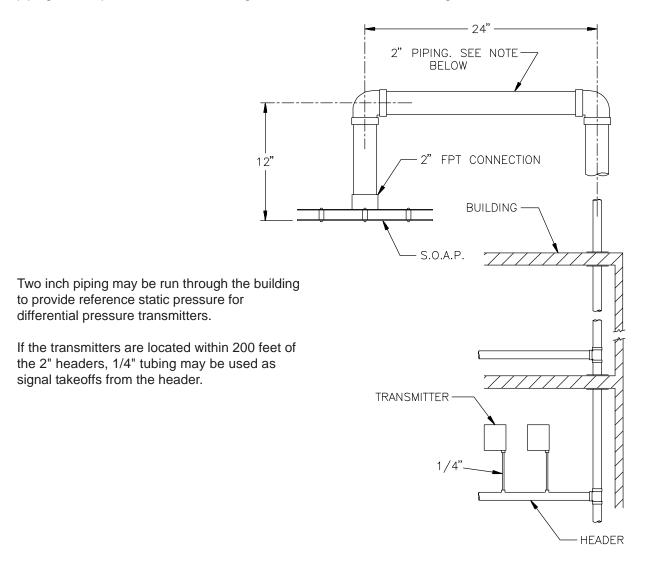
CAUTION: After signal piping is completed, signal lines must be leak tested prior to operation.
