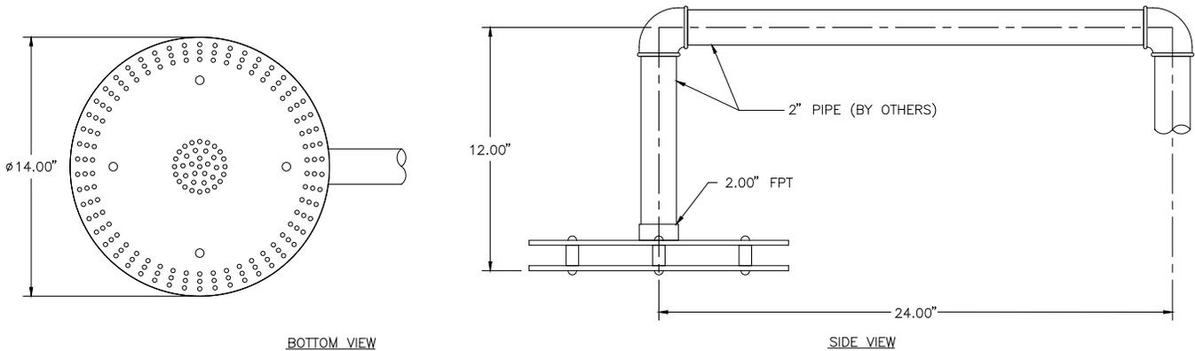
Provide for the room or space static pressure indicating or controlling systems an outdoor static pressure sensor constructed of 10 ga. Type 316 stainless steel with a 2" diameter FPT connection.
