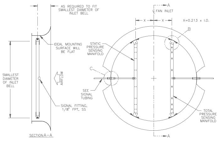
Note: When placing an order for a VOLU-probe/FI, be sure to state the minimum fan inlet diameter, not the fan model number nor the probe length. (The probe length will be approximately 0.905 the minimum inlet diameter for standard configurations.
