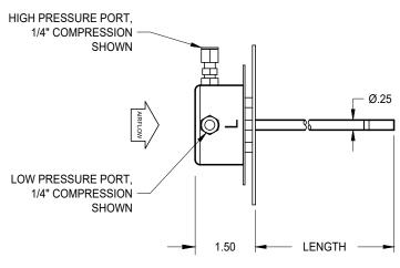
(Note: 3" length standard, available up to 8" in 1" increments. Length should include louver depth plus 2")
